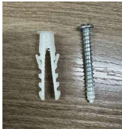
Fig 12. Anchorage used for pull down test
