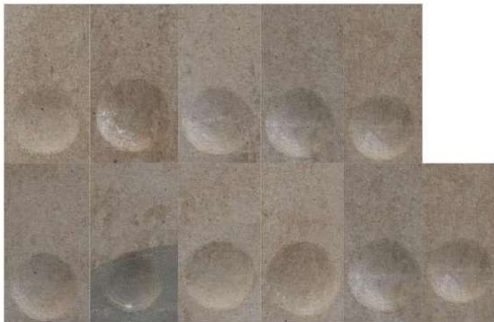
Fig 3. Locations of small hard body impact for surface damages (above)
