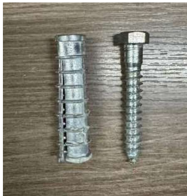
Fig 16. Anchorage used for wash basin test
