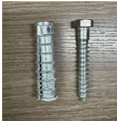
Fig 14. Anchorage used for wash basin test
